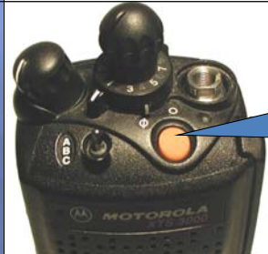
EMERGENCY ACTIVATION BUTTON
